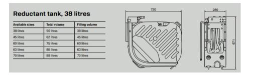
Application Plastic tank to fit in steel box
