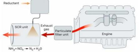
A chemical process is started when reductant, a urea and water mixture, is injected into the exhaust gas stream. During injection, the water evaporates and the urea breaks down to form ammonia. The ammonia then reacts with the nitrogen oxide gases in the catalytic converter and forms harmless products such as nitrogen gas and water.
